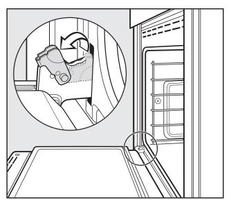
■ Slowly shut the door until the protruding clamps stop the movement. Pull the door upward.
