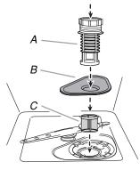
A. Main filter B. Metal strainer C. Fine filter
