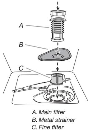
**NOTE:** The dishwasher should not be operated without the filter assembly installed. Improper replacement of the filter assembly may reduce the performance level of the appliance and may damage dishes and utensils.
