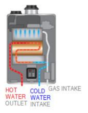
water fixture shuts off, cold water stops flowing into the tankless water heater and the flame extinguishes. The tankless water heater is now off until the next time hot water is needed.
