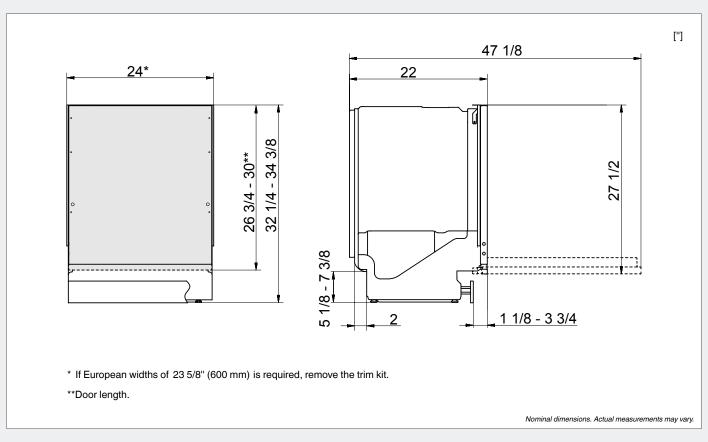
It is important that you read through and follow the instructions and directions below. Conduct installation and connection in accordance with the separate installation instructions.
