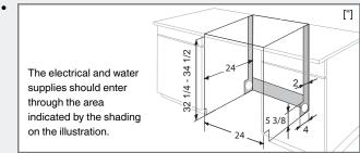
Make sure the area on which the dishwasher is to be installed is firm. Adjust the adjustable feet so that the dishwasher is level.
