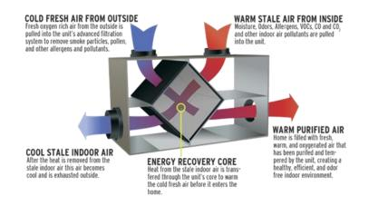
To maintain the ERV system, an access panel has been installed. Filters are to be cleaned every 3-6 months depending on living conditions (excess pet hair, dust etc.). <u>We recommend</u> <u>maintenance be done on the ERV unit by a mechanical professional on a quarterly basis.</u>
