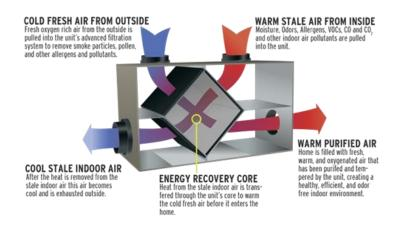
To maintain the ERV system, an access panel has been installed. Filters are to be cleaned every 3-6 months depending on living conditions (excess pet hair, dust etc.). <u>We recommend maintenance be done on the ERV unit</u> by a mechanical professional on a quarterly basis.
