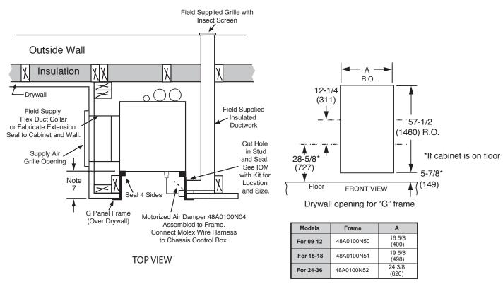
Figure 11: Cabinet with "G" Panel Frame and Optional Outside Air Duct (Field Fabricated)
