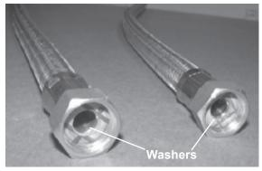
Step 3: Attach AHH or AHU hoses to the Chassis. Check the swivel ends of the hoses (Figure 21). Washers must be in the hose for water tight connection. Slide the chassis part way into the cabinet. Match the WATER IN (supply) hose to the WATER IN tube on the chassis and the WATER OUT (Return) hose to the WATER OUT tube. Position hose toward chassis, use gentle loop- see bend radii Table 7. Hand tighten hose.
